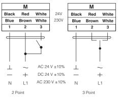
↑ Connect via safety isolating transformer
